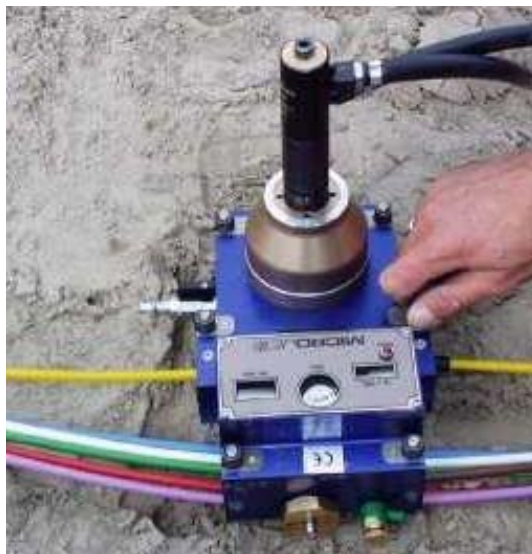
Figure 3. Jetting micro-cables in tandem
